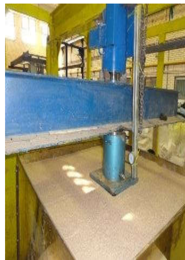
Figure 4. Plate load test before and after loading
