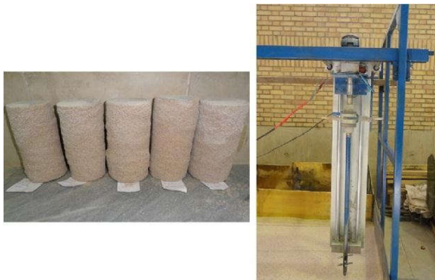
Figure 5. Deep soil mixing device and sample of columns
