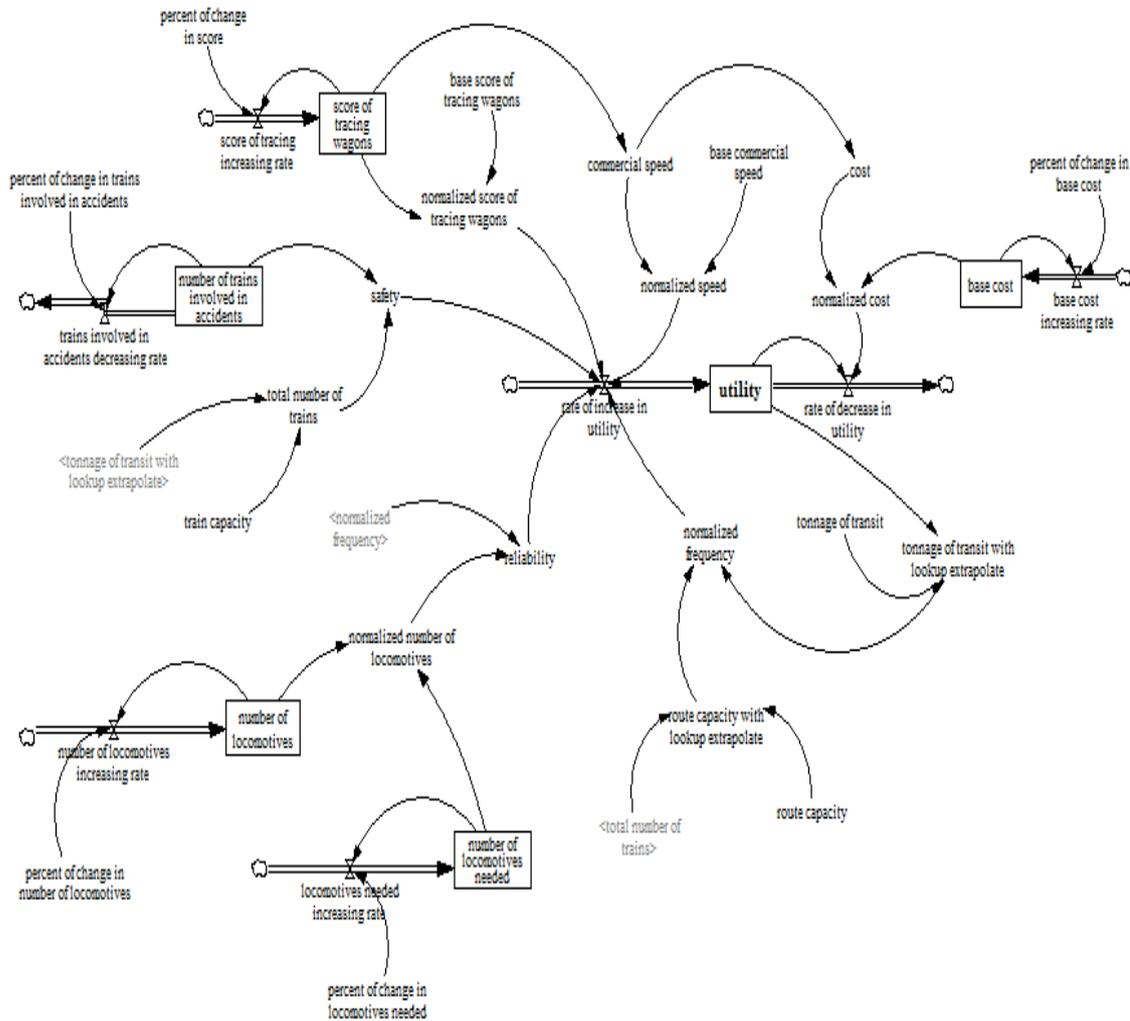
Figure 3. The stock and flow diagram of the rail transit system
