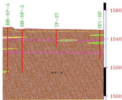
Figure 6. Soil layers in the selected parking area
