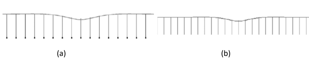
Figure 15. Lateral view of the track deformation (deformation scaled \times 100 ): (a) Computational tool; (b) ANSYS
