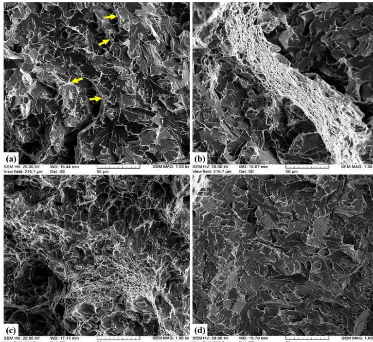
Figure 12. Fracture surfaces of a GS20Mn5 steel specimen austenitized at  $930^{\circ}\text{C}$  and cooled at different rates (a) cooled by still air; (b) cooled by forced air with 50% humidity; (c) cooled by forced air with 70% humidity; (d) cooled by forced air with 90% humidity (small dimples indicated by arrows)
