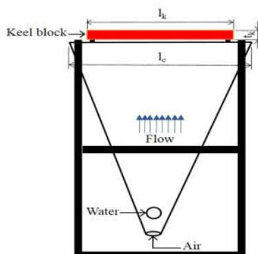
Figure 2. Schematic view of the cooling channel
