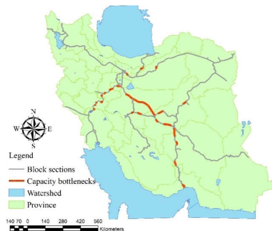
Figure 4: Identification of the capacity bottlenecks in Iranian railway network
