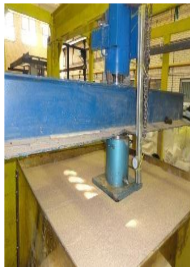
Figure 4. Plate load test before and after loading
