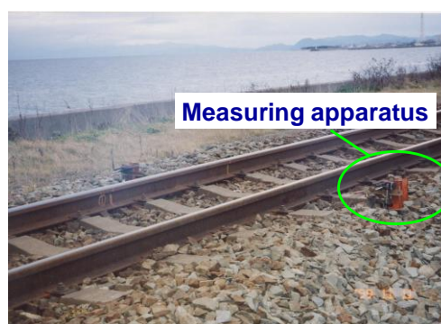
Figure 3. Track site for measurements of track settlement
