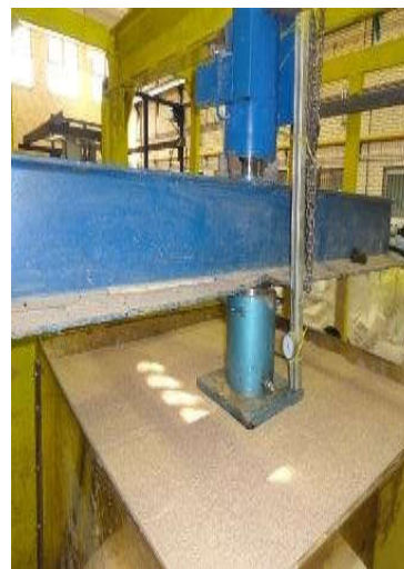
Figure 4. Plate load test before and after loading
