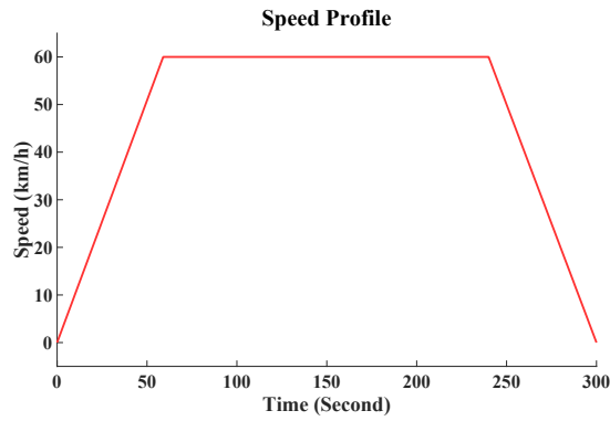
Figure 8. Sample of an electric train speed profile.
