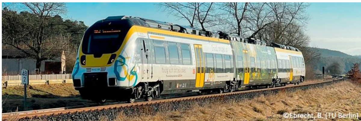
Figure 1. The Alstom BEMU test train [5].
