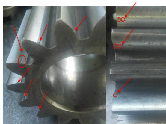
Fig. 1 Real pitting in the gear power transmission system of a locomotive.
