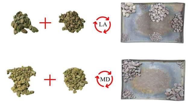
Figure 3. Images of graded aggregates before and after LAA and MDA tests.
