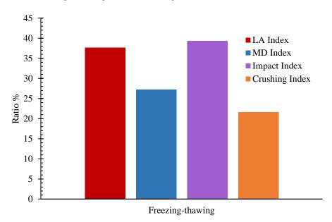
Figure 6. Changing rates of evaluation indices under freeze-thaw conditions compared to normal temperature
