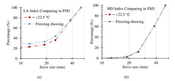
Figure 5. Grading curves of the ballast aggregate breaking index for freeze-thaw conditions compared to normal conditions after performing tests: (a) Los Angeles abrasion, (b) Micro-Deval abrasion
