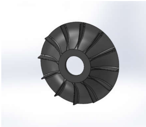
Figure 5. Radial Blade with 12 Blades
