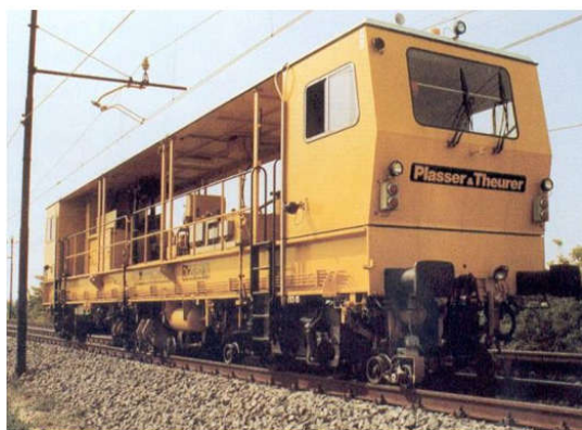
Figure 7. “Dynamic Track Stabilizer (DTS)”
