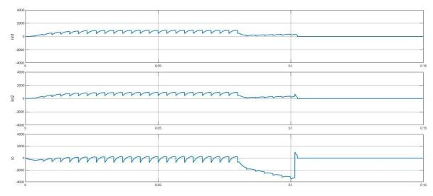
Fig 8. The input currents of 1<sup>st</sup> inverter module (up), 2<sup>nd</sup> inverter module (middle) and DC link capacitor (low) for DC link short circuit
