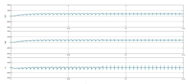
Fig 10. The input currents of 1<sup>st</sup> inverter (up), 2<sup>nd</sup> inverter (middle), and DC-link capacitor (low) for DC link open circuit
