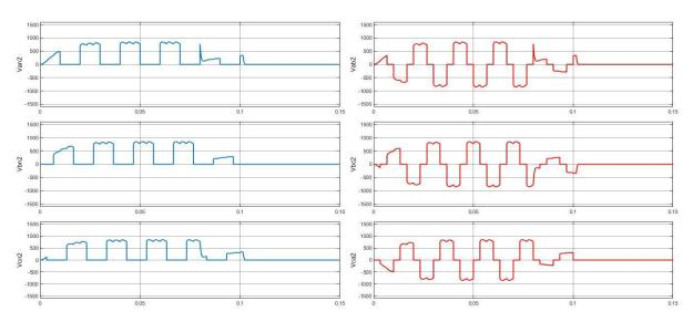
Fig 9. The output voltages of inverters (left: phase voltages, right: line voltages) for DC link short circuit
