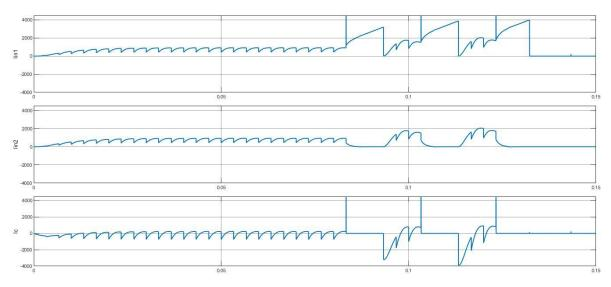
Fig 12. The input currents of faulty (up), non-faulty (middle) inverter, DC-link capacitor (low) for switches short circuit
