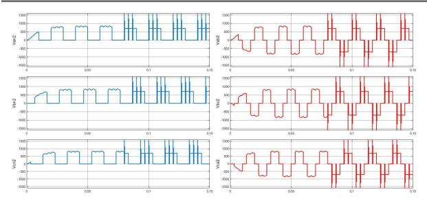
Fig 11. The output voltages of inverters (left: phase voltages, right: line voltages) for DC link open circuit
