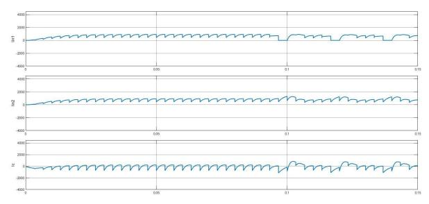
Fig 14. The input currents of faulty (up), non-faulty (middle) inverter, DC-link capacitor (low) for switches open circuit
