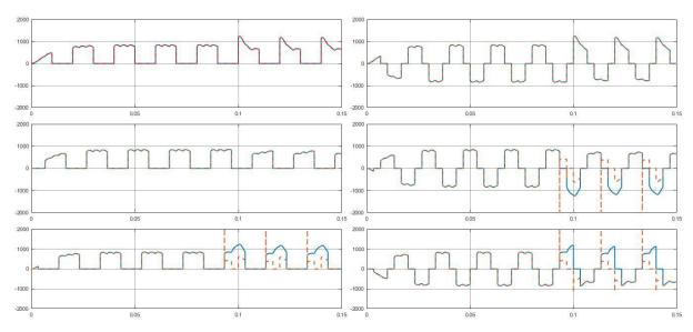
Fig 15. The output voltages of faulty(red) and non-faulty (blue) inverters for switches short circuit
