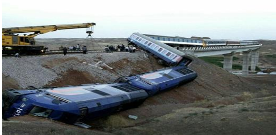
Figure 1. Derailment of the train due to rail removing (Iran 2020)
