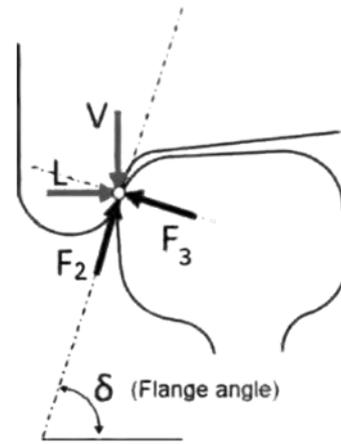
Figure 1. Schematic of forces in flange connection [6]
