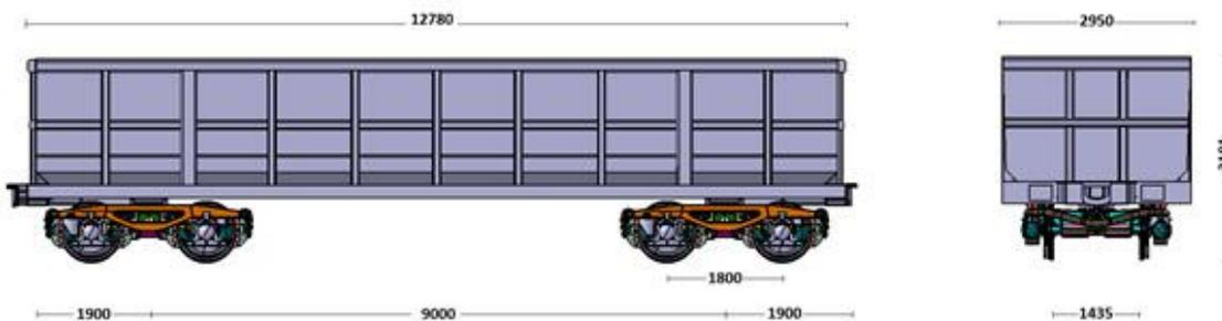
Figure 3. Specifications of the long-edged open cargo wagon[8]
