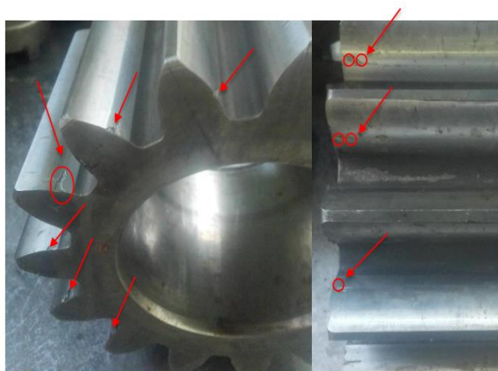
Fig. 1. Real pitting in a gear power transmission system of a locomotive
