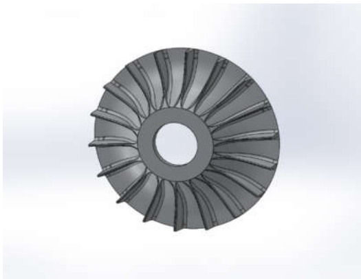
Figure 4. Radial Blade with 18 Blades
