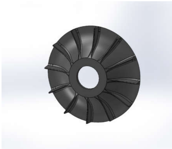
Figure 5. Radial Blade with 12 Blades
