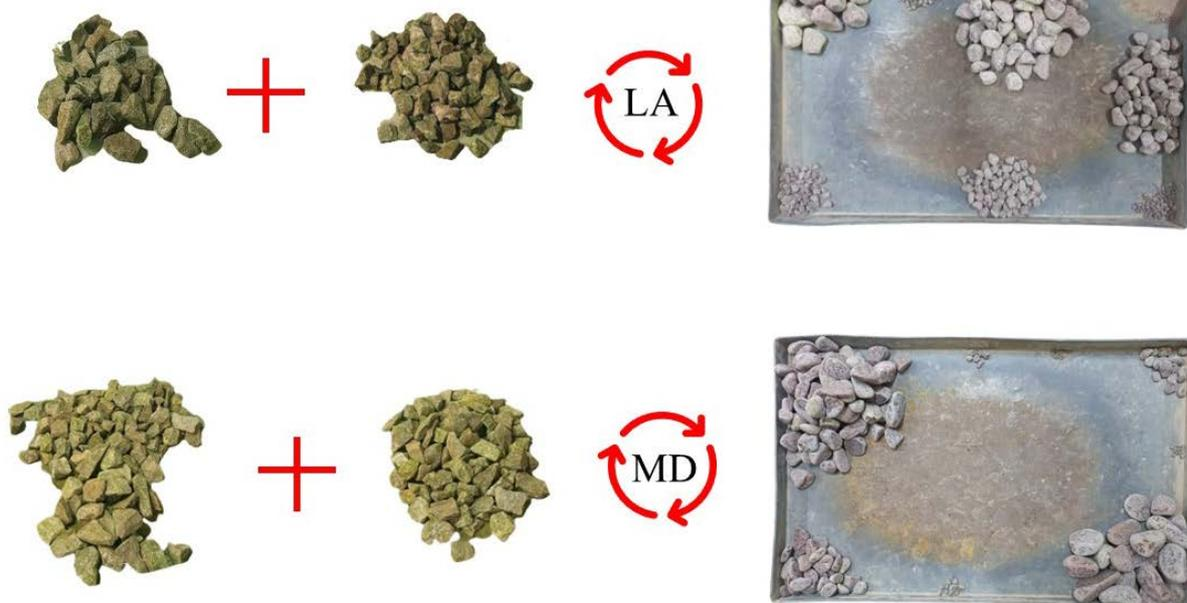
Figure 3. Images of graded aggregates before and after LAA and MDA tests.
