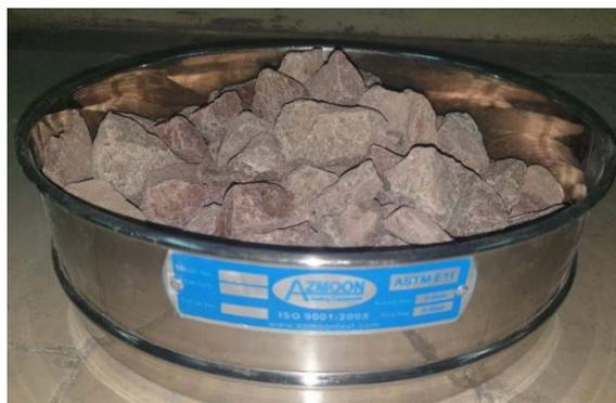
Figure 1. Samples of ballast aggregates
