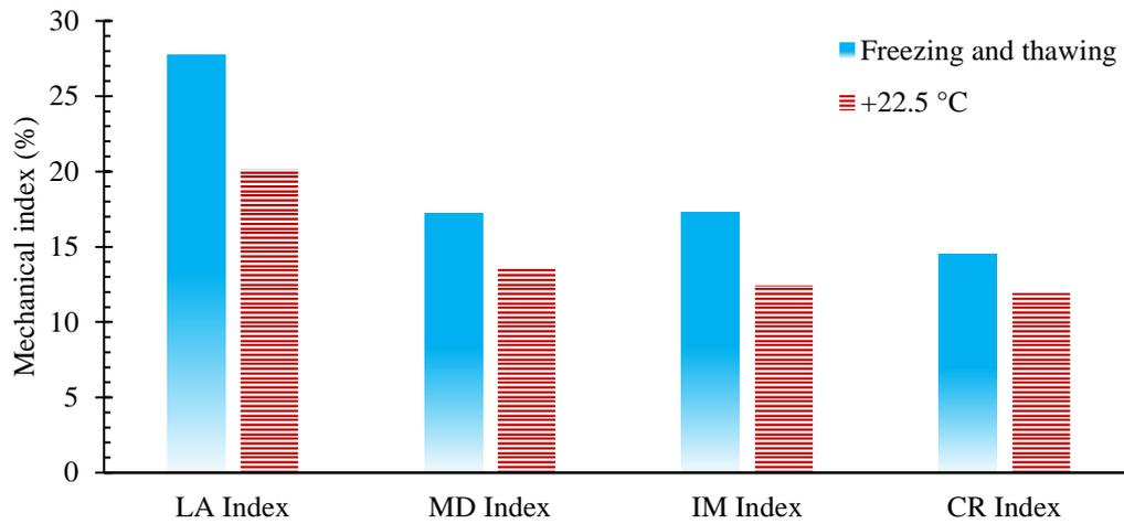
Figure 4. Evaluation Indices obtained from freezing-thawing test
