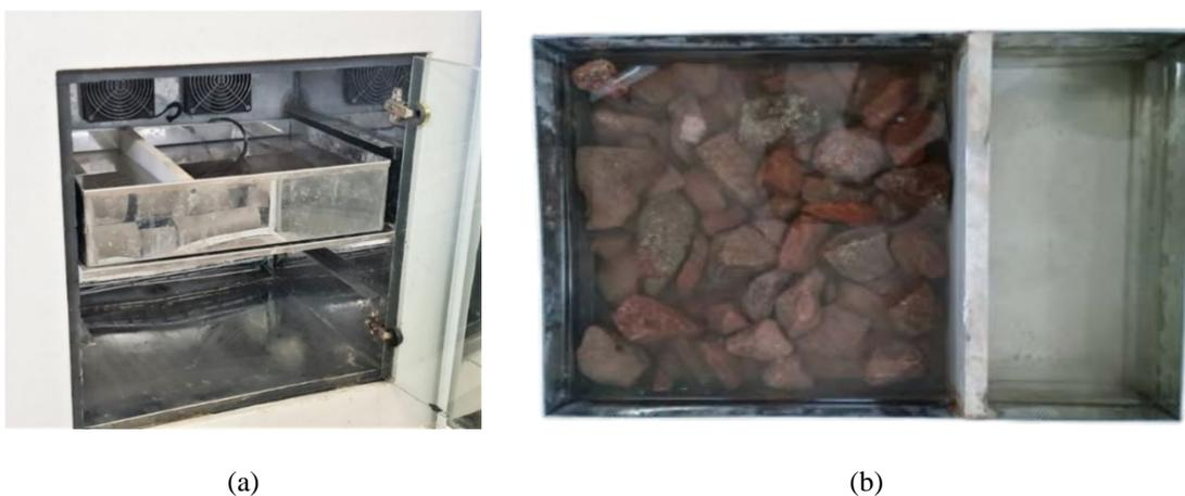
Figure 1. Freeze-thaw test setup: a) Freezing-thawing machine, b) Ballast aggregates in chamber
