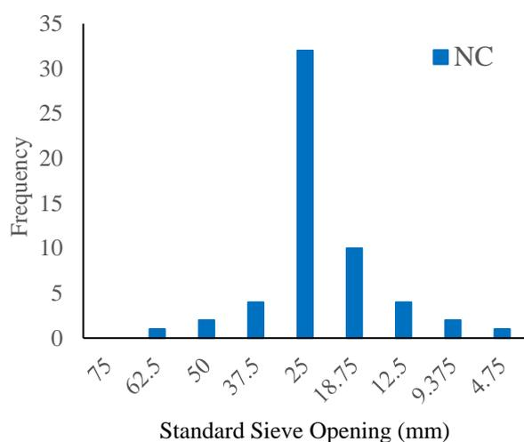
Figure 6. Frequency of Flying Aggregates per Sieve
