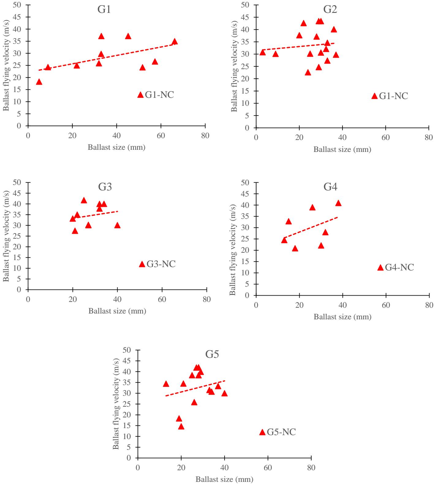
Figure 4. Variation of ballast flight velocity regard to aggregate size for different ballast gradations in non-compacted (NC) States
