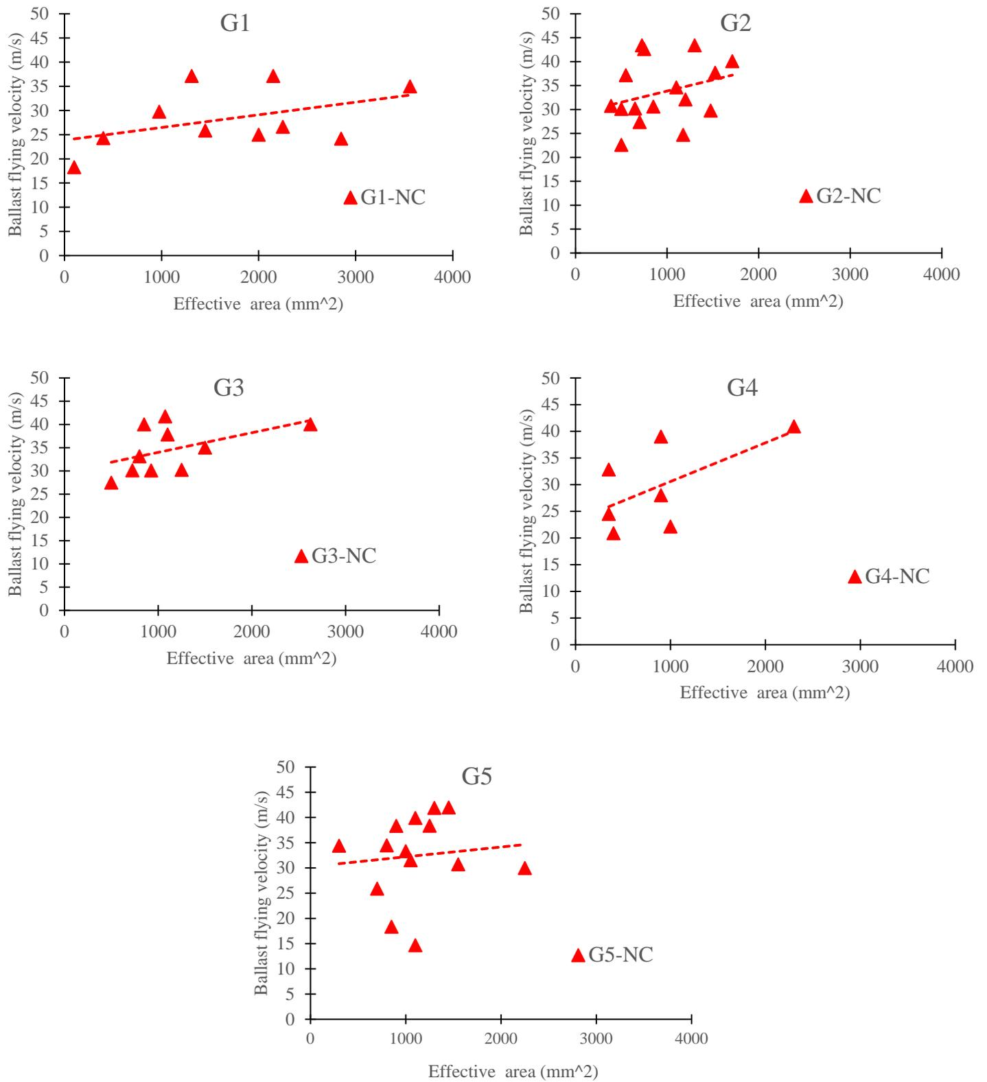
Figure 2. Variation of ballast flight velocities against effective area of flying aggregates
