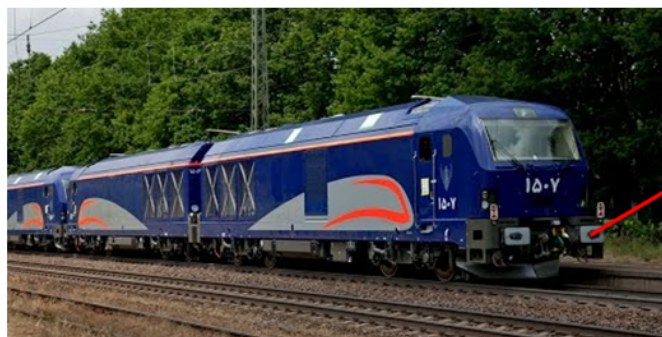
Figure 3. Front end energy absorbing equipment in IrSa locomotive [1]
