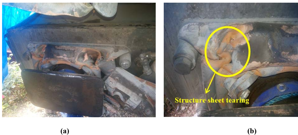
Figure 4. (a) Destruction of the crash element and buffer (b) rupture of crash element sheets from the corners due to the shear stress concentration [1]
