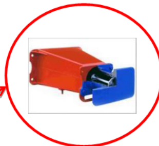
Figure 3. Front end energy absorbing equipment in IrSa locomotive [1]
