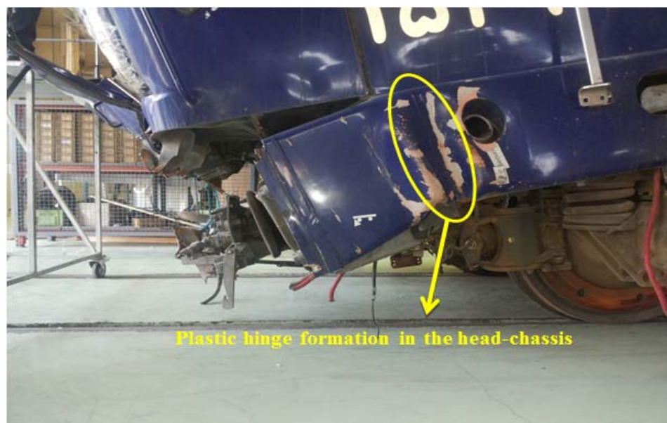
Figure 5. The damage to the front parts of the locomotive, including a buffer, the crash element and head-chassis [1]
