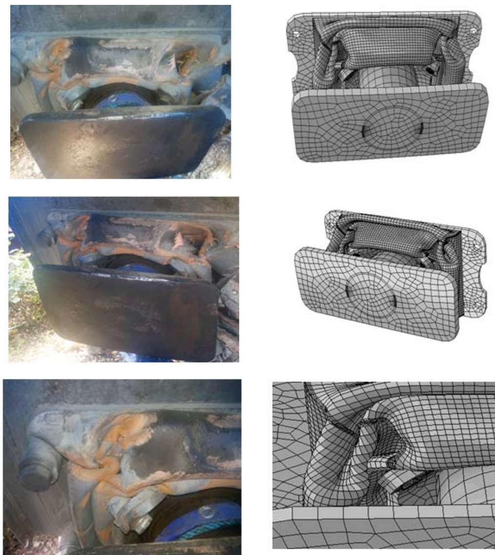
Figure 11. A comparison of the numerically simulated deformation and the real crash results
