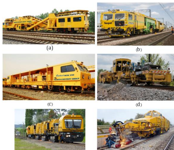
Figure 2: Equipment of maintenance operations: (a) ballast cleaner, (b) ballast tamper, (c) track stabilizer, (d) ballast regulator, (e) rail grinder, (f) rail welding machine.
