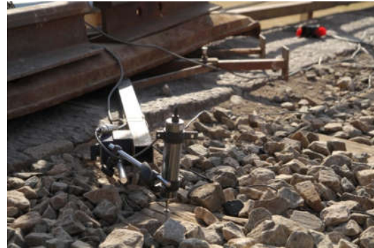
Figure 4: LVDT mounted on sleeper to determine the exact speed and location of test train axles
