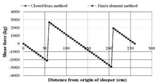
**Figure 2.** Shear force of sleeper
