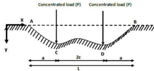
**Figure 1.** Sleeper as a beam with finite length caused by two loads
