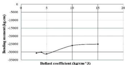
Figure 10. Bending moment in the middle of sleeper
