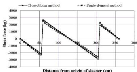
**Figure 7.** Shear force of sleeper
