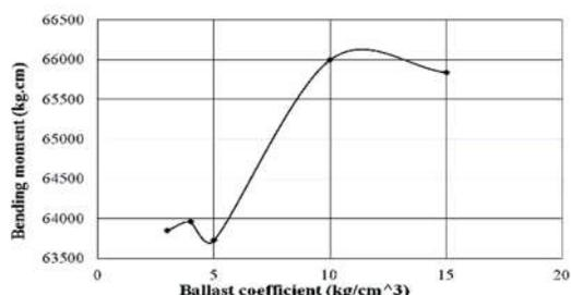
Figure 11. Bending moment in the rail seat
