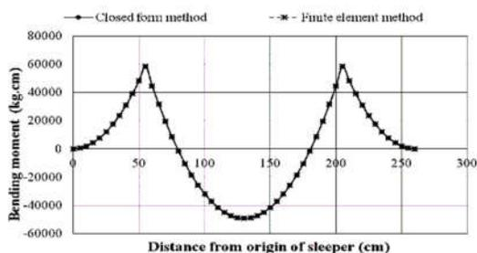
**Figure 3.** Bending moment of sleeper
