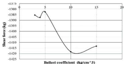
Figure 12. Shear force of sleeper in distance of 20 cm from rail seat
