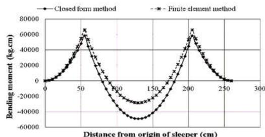
**Figure 6.** Bending moment of sleeper
