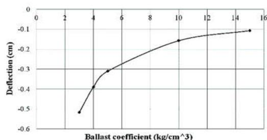
**Figure 9.** Deflection of sleeper in the rail seat
