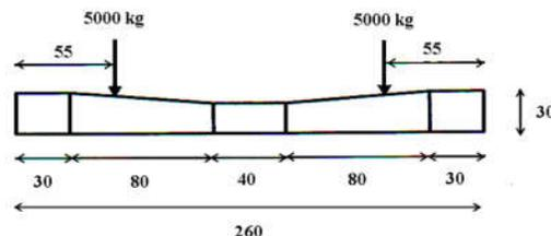
**Figure 4.** B70 concrete sleeper (Geometric dimensions in centimeters)
